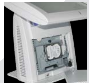
Accessible hard disk and USB
